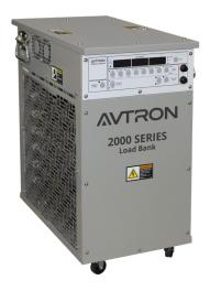
The Avtron Model 2705 is a resistive, AC load bank at 100kW @ 240/480V, 3P, UL rated.
