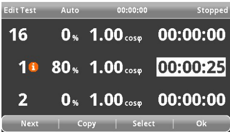
Figure 4-22 A warning is shown if the connected load bank cannot apply the load.
